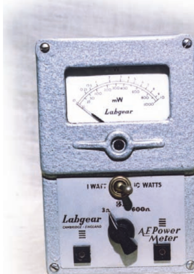
● Fig. 2: The Labgear audio frequency power meter which appears to have been offered as a kit (see text).
