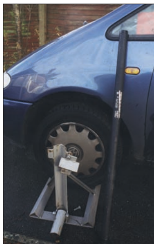
● Fig. 1: An ideal partnership - the Funktechnik 10m telescopic mast shown packed into its integral carrying tube (which also forms the base of the mast) and the PW 'Tenna-Tourer' drive-on mast base (see text).
